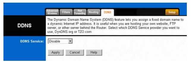
The Router offers a Dynamic Domain Name System (DDNS) feature. DDNS lets you assign a fixed host and domain name to a dynamic Internet IP address. It is useful when you are hosting your own website, FTP server, or other server behind the Router. Before using this feature, you need to sign up for DDNS service with one of two DDNS service providers, DynDNS.org or TZO.
